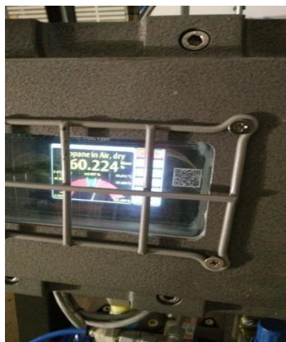
Figure 4. Inline Propane Ratio Measurement Device at SEAP.
